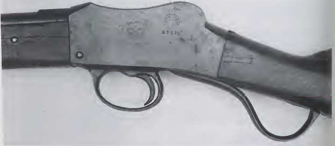
Figure 35 The Western Australian Government ownership stamp impressed on the left side of the body of the Francotte Martini rifle discussed in Figure 33. This mark, along with the Francotte patent mark were impressed by the factory at the time of manufacture. (Photo D. Elford).
